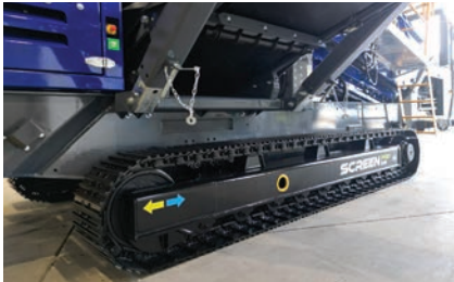
Chassis Riser - Increase ground clearance by and allows for higher stockpile capacities.
