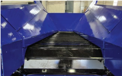
Apron Feeder - for heavier, coarse feed material.
