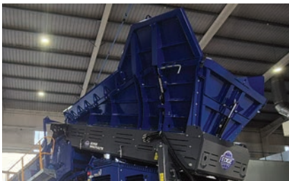
Hydraulic Hopper Extensions - increased hopper capacity and loading target area.
