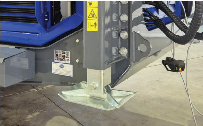
Hydraulic Chassis Jack Legs - supports the feeding of heavier, coarse feeds.
