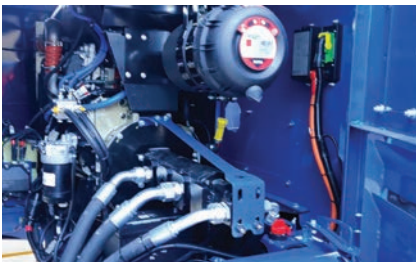
T4F / STAGE V- CAT 3.6 10Kw (134HP) (LRC option also available)
