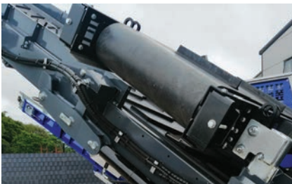
Magnetic Head Drum / Overband Magnets - enables ferrous metal recovery.
